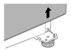
Loosen the 2 bolts and the Phillips head screw and remove the middle hinge bracket from the refrigerator housing. Set the parts aside.
