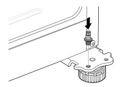
**6** Using a 3/8 in. socket wrench with a 2-inch extension, loosen the 2 bolts on the bottom hinge bracket. Use a Phillips screwdriver to loosen the screw.
