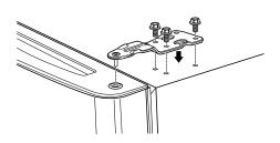
Place the top hinge on top of the freezer door and line up the hinge with the holes on top of the refrigerator. Use the three bolts to fasten the hinge.
