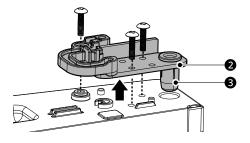
Move the bracket to the opposite side of the door and insert the hinge pin sleeve. Reverse the hinge lever 4 by flipping it over. Place it on top of the bracket, and tighten both down with the screw. Then insert the remaining 2 screws to tighten the bracket to the refrigerator door.
