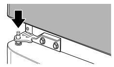
Place the top hinge on top of the freezer door and line up the top hinge with the holes on top of the refrigerator. Use the three bolts to attach the hinge.
