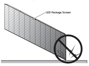
2 If the product is tilted towards the edge of the LED package screen after the brackets on the corners are removed, the bottom (corner) of the product may be damaged.
