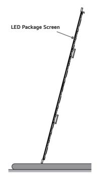
3 Place the product with the LED package screen facing down. To protect the screen, lay the protective pad in the box on the floor.
