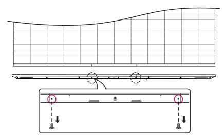
2 Push the lock-structured knob back and detach the bottom front cover downwards.
