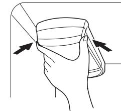
**3** Pull the water filter downward and turn it counterclockwise before pulling it out.
