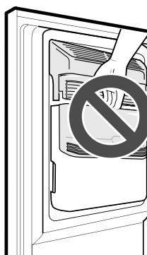
**1** To detach, lift the ice storage bin slightly and pull it out as shown in the figure.
