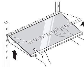
**3** To assemble, tilt the front of the shelf up and guide the shelf hooks into the slots at a desired height.
