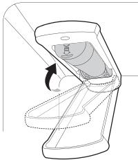
**6** After the water filter is replaced, dispense 2.5 gallons of water (flush for approximately 5 minutes) to remove trapped air and contaminants from the system.
