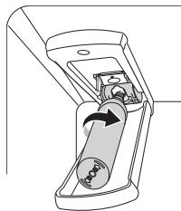
**5** Close the water filter cover. The cover will click when closed correctly.
