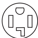
4-Wire Receptacle (14-30R)
