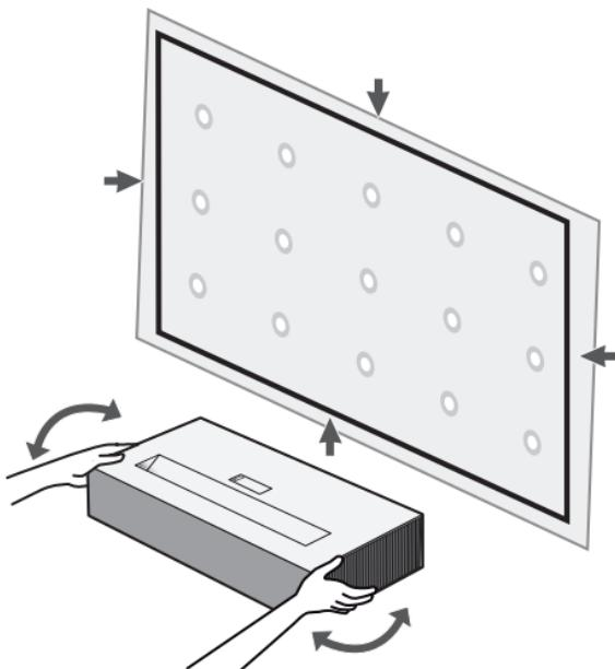
**3** To adjust the focus of the image, slowly adjust the focus ring to the left or right while looking at the top center of the screen. You can adjust the focus most effectively when the left and right screen are balanced. When adjusting the focus on the screen, do not let the product shake.
