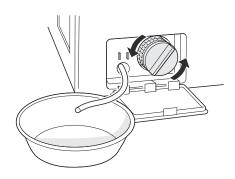
**5** Clean the pump filter and opening.
