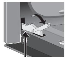
Figure 16: Unlocking door hinge
