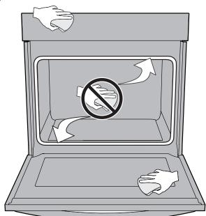
Figure 8: Clean around the oven door gasket
