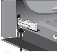
Figure 15: Door hinge locked
