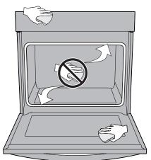
Figure 10: Clean around the oven door gasket
