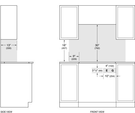
NOTE: Shaded area above countertop indicates minimum clearance to combustible surfaces, combustible materials cannot be located within this area.
