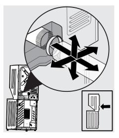
An exhaust hood positioned to line up with the dryer exhaust can be installed directly through the outside wall. To exhaust to the side or down, add an 8 inch (20.3 cm) length of standard 4 inch (102 mm) diameter duct and a 90° elbow.
