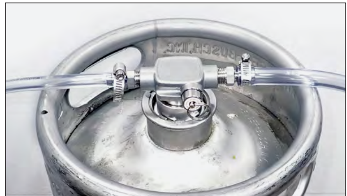
FIG. 10. Installed and connected taper. Be sure the hose clamps are tightened to prevent links.
