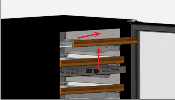
FIG. 1. Lift and pull the wine rack forward.
