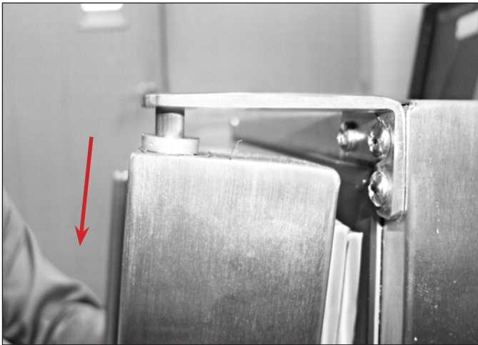
FIG. 3. Lower the door off the top hinge.
