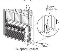
After the air conditioner is installed, measure the curtain panel on each side and cut the adhesive-backed heatproof foam to fit each panel. The size of the panels may differ. Remove the backing from the heatproof foam and attach the foam to the curtain panels.
