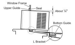
2 Extend the guide panels to fill the window opening and use 4 type B screws to secure them to the window
