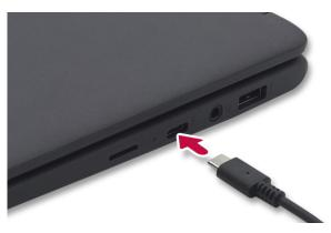
2 Open the LCD and check the charging state.
