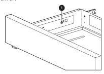
3 Locate the glide lever on each side of the drawer. Push down on the left glide lever and pull up on the right glide lever.
