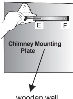
Screw the chimney mounting parts into Ø 8mm sized wall plugs on E,F points which are provided with your product.
