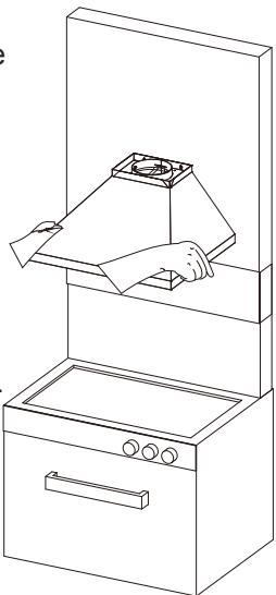
Then fix the body on (A, B) holes to the wall using the screws.
