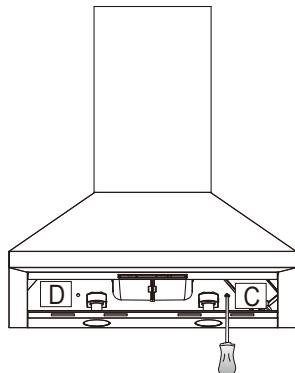
**NOTE:** If the hood seems to be tilting, slightly loosen the screws that are used on the hanging parts at the top and straighten until the hood is vertical.
