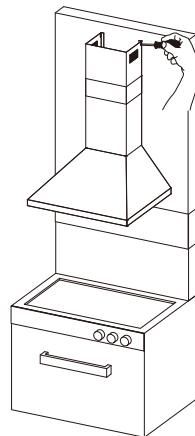
Screw internal chimney on chimney fixing sheet, fixed over upper corner of external chimney.
