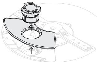
Remove the drain filter and the filter plate from the bottom of the drawer. Use a sponge to remove any remaining water from underneath before replacing.
