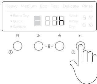
Press and hold **►||** until **1h** appears in the display to enter **DELAY START** mode.
