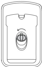
Turn the plug anticlockwise and remove.
