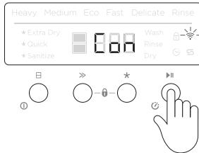
Press and hold ►II to connect to the Wi-Fi network.
