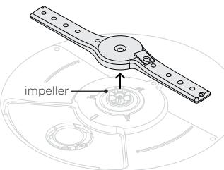
Lift the spray arm off the impeller. Shake to dislodge any loose particles, rinse under running water and wipe with a damp cloth.
