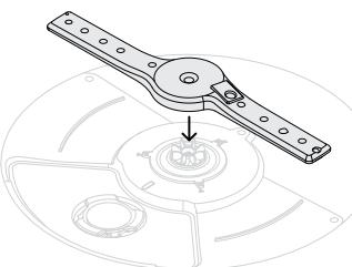
Place the spray arm to the impeller. Ensure the arm rotates freely when refitted.
