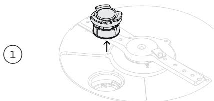
Twist the drain filter counter-clockwise and lift to remove.
