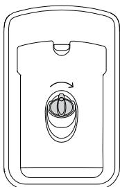
Refit the plug, turning clockwise until secure.
