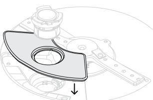
Push the drain filter plate back onto the tub ensuring there are no particles in the recess.
