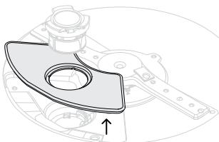
With the drain filter removed, carefully lift the drain filter plate up and out. Clean under hot soapy water and rinse thoroughly.
