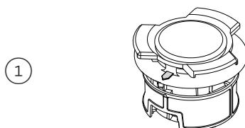
Click the drain filter mesh back onto the holder and twist until the arrows on the mesh and holder align.
