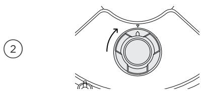
Push the drain filter back into the tub and rotate clockwise until the arrows on the filter and base of the drawer align.
