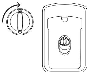
Refit the cap, turning clockwise until secure.
