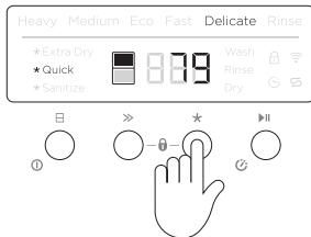
Press **★** to scroll through the available wash modifiers. The selected wash modifier indicator will illuminate on the display.
