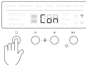
Press and hold ① to save and leave the menu after Wi-Fi is connected.
