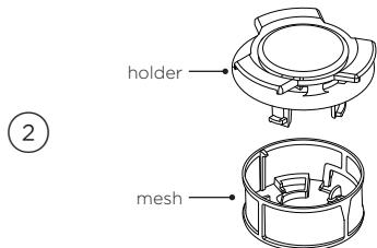
Separate the holder and the mesh by pinching one side of the mesh and pulling.
