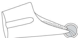
Place the salt into the salt container and carefully pour into the reservior.
