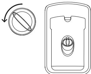
Turn the cap anticlockwise and remove.
