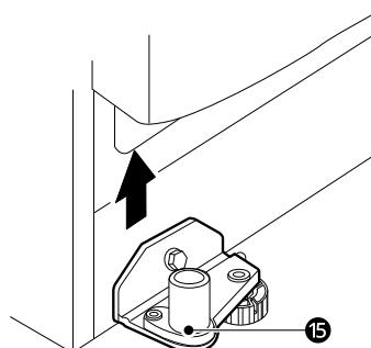
**Removing the Refrigerator Door**
