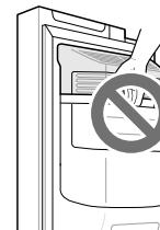
**1** To detach, lift the ice storage bin slightly and pull it out as shown in the figure.
