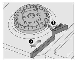
■ Place the wire brush on the right side of the burner (1.) and brush off the baked-on deposits from the ignitor (2.).
