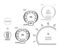
2 Select a number in the element power settings to adjust the power level. If a power level is not selected after 10 seconds, the element's power level remains the same.
