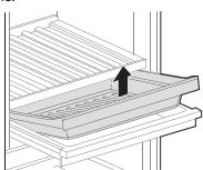
Keeping both levers 2 pressed, lift the drawer support slightly and remove it from the rail.
