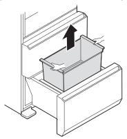
The auto-lift device is at the bottom of the drawer. Hold the inner edge of the device with both hands and pull it up.
