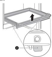
To assemble, hook the drawer support on the rails located on both side and press it down until you hear snap sound.
