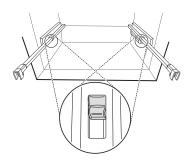
Angle the drawer into the frame and set it in place.
