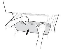
7 Insert the supplied hole cover into the groove at the bottom of the drawer.
