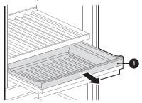
Lift the drawer straight up and out of the frame.
