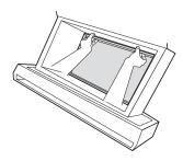
Hold the top of the auto-lift device with both hands and remove it from the bottom drawer.
