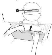
Hold the middle of the cover and lift it slightly into the groove.
