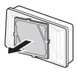
To reset the filter replacement period, press the **Air Filter** button on the control panel until the icon on the control panel turns off.
