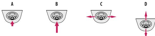
**A (Power on):** Press the joystick button once with your finger to turn on the monitor.
