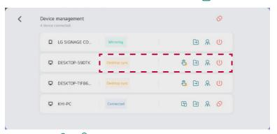
3 When the icon changes to  $\bigcirc$   $\rightarrow$   $\bigcirc$ , you can control the Interactive Digital Board from the device.
