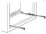
**2** Line up the bottom edges on the sides of the drawer support with the groove in each rail and then lower the support until it clicks into place.
