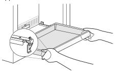
Keeping both levers pressed, lift the drawer support slightly and remove it from the rail system.
