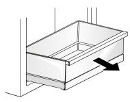
Lift the empty drawer slightly to remove it from the support.
