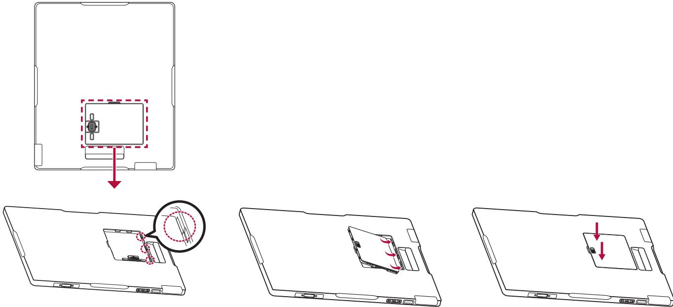
1 Check the direction of the holes located inside the detector.
