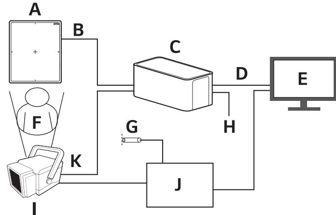
Main Cable: Connects the control box to the detector.
