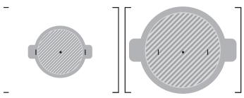
Figure 8: Zone two min / max pan size
