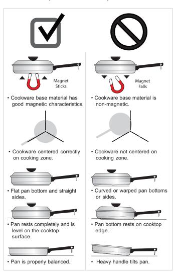
Figure 6: Pan sensing conditions
