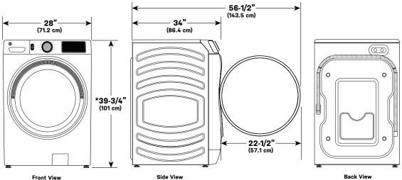
\*With leveling legs retracted: 39-3/4" (101 cm). With leveling legs fully extended: 40-5/8" (103.1 cm).
