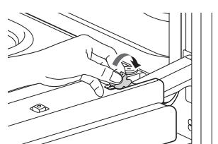
**3** Close the door to 30 degrees **1** (you will feel the door stop). The hinge locks will contact the oven frame.
