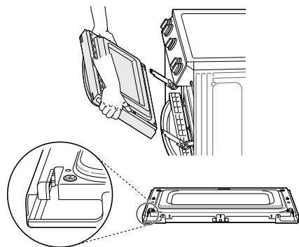
**4** Press the hinge release buttons **2** on either side of the door.
