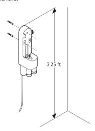
Attach the charging station to the wall with the wall anchoring screws.
