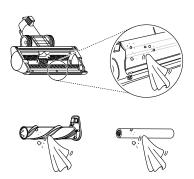
7 Slide the brushes back into the nozzle and rotate the cover back into place. Turn the cover lock clockwise to lock the cover.
