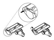
Pull the brush cover forward and pull the main brush out.
