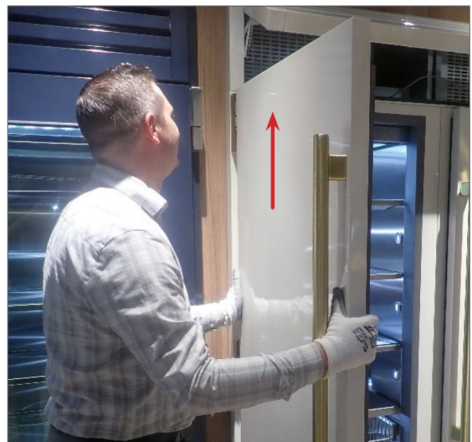
FIG. 3. Remove the door.
