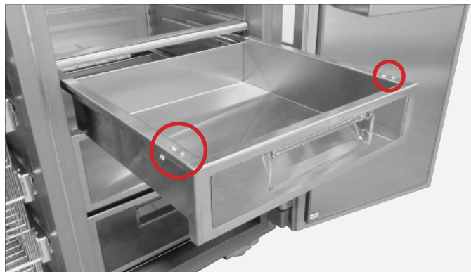
FIG. 5. Drawer slide screw locations..
