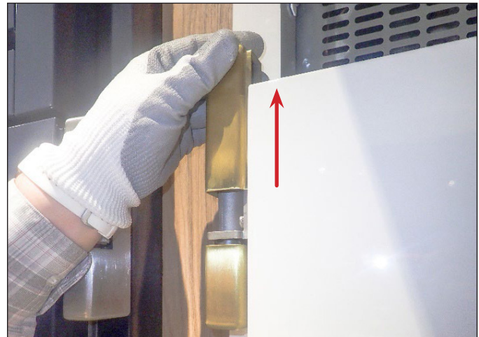
FIG. 2. Remove the hinge covers.
