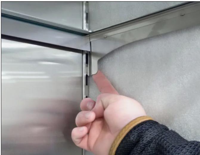
FIG. 6. Push the bottom tab inward.
