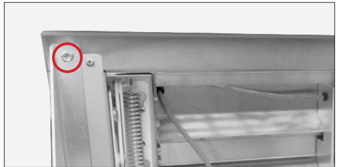
FIG. 8. Bracket screw location. Other bracket not shown.
