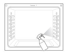
Spray or pour the remaining water (8 oz or 240 ml) onto the bottom center of the oven cavity. The indentation on the oven bottom should be fully covered to submerge all soils. Add water if necessary.
