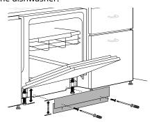
Attach a custom toe kick. If needed, use a saw to cut a notch in the top of the custom toe kick to provide clearance for the cabinet panel when opening the door.
