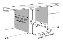
To allow for proper clearance of plumbing and electrical, use the template included with the literature to determine the clearance on the side of the cabinet where the cabinet meets the back wall. Using a 2 1/2" diameter hole saw, drill a hole in the target area as shown on the template.
