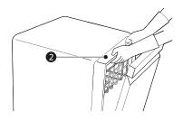
Align the dishwasher with the opening. Make sure the water supply line and power cord extend smoothly without kinks or bends.
