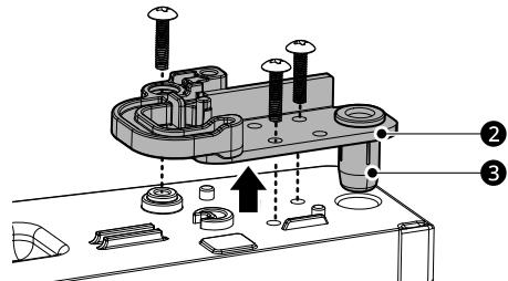
**6** Move the bracket to the opposite side of the door and insert the hinge pin sleeve. Reverse the hinge lever **4** by flipping it over. Place it on top of the bracket, and tighten both down with the screw. Then insert the remaining 2 screws to tighten the bracket to the refrigerator door.
