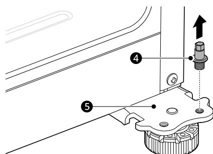
**5** Reattach the bottom hinge pin to the opposite side of the bottom hinge bracket.
