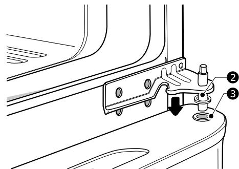
**3** Hold the door in place and line up the hinge with the holes in the refrigerator housing.
