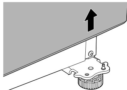
**3** Loosen the 2 bolts and the Phillips head screw and remove the middle hinge bracket from the refrigerator housing. Set the parts aside.
