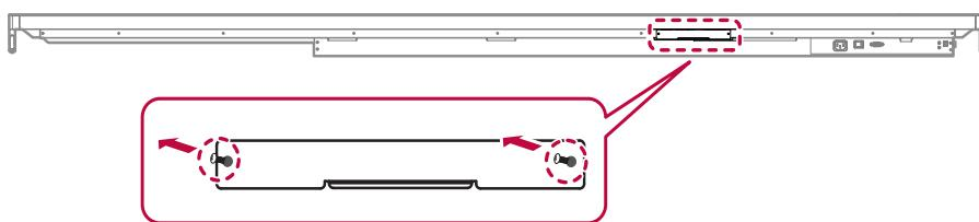
2 Following the direction of the arrow, insert the Wi-Fi module fully into the slot.
