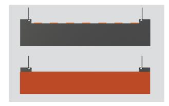
5. For a toe kick depth of 1 9/16 - 3 15/16", align the custom panel along the lower edge of the toe kick mount.
