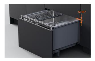
5. Slot panel onto dishwasher. Check that the gaps between the panel and adjacent cabinet doors are a minimum of 1/16". Check that the gap between the top and bottom drawer panels is a minimum of 5/16" for ventilation.
