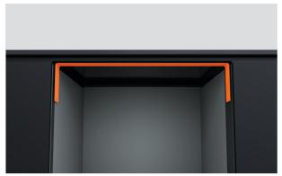
**3.** Apply tape to top edge of cabinet ensuring it is centred and set back 3/8" from the front edge.
