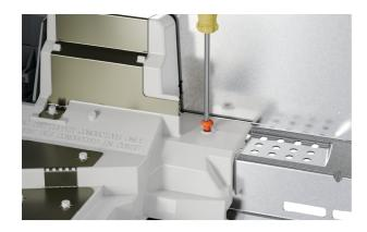
**3.** Remove the screw securing the cover and set aside.
