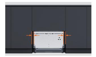
1. Measure the distance from the adjacent cupboard doors to the edges of the door bracket.
