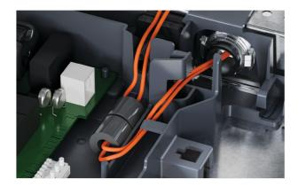
**8.** Fit a suitable cable clamp for the conduit through the metal knock-out.
