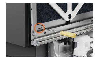
**4.** Fit a screw in each chassis slot to secure to the cabinet. Partially tighten screws ensuring adjustments can be made.
