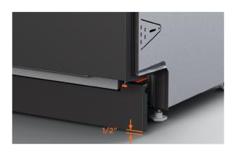
**4.** Snap off the top tabs. Slide the jig and toe kick along the T rails into position. Ensure there is a 1/2" gap between the toe kick and the floor.
