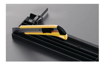
**3.** Score the toe kick on both sides with a box cutter on a protective surface.
