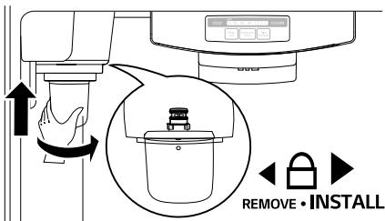
**5** After the water filter is replaced, dispense 2.5 gallons (10 liters) of water (flush for approximately 5 minutes) to remove trapped air and contaminants from the system.
