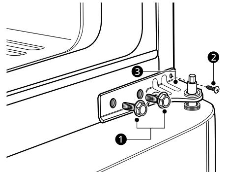
**2** Lift up the refrigerator door slightly and remove it. Set the door aside on a non-scratching surface.
