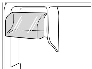
**2** To replace the dairy bin, slide it in above the desired support slots and push down until it stops.
