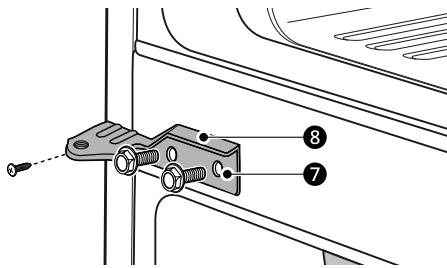
**10** Place the refrigerator door down over the bottom hinge pin on the bottom hinge bracket.
