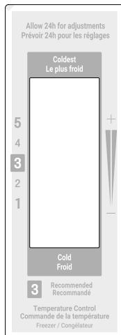
The freezer control should ship set to the middle setting (number 3). Wait 24 hours before adjusting the freezer compartment temperature. Roll the knob to set the freezer temperature as you desire. ALWAYS wait 24 hours after any adjustment to reach the desired temperature.
