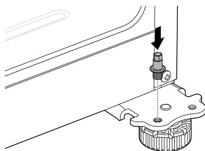
**6** Using a 3/8 in. socket wrench with a 2-inch extension, loosen the 2 bolts on the bottom hinge bracket. Use a Phillips screwdriver to loosen the screw.
