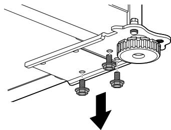
**7** Remove the bottom hinge bracket from the right side of the housing.
