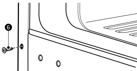
**9** Flip the middle hinge bracket **7**. (The flange **8** will now be on top.) Position it on the left side of the refrigerator and reattach it with two bolts and a Phillips-head screw.
