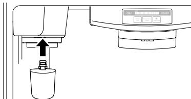
**4** Push the water filter up into the filter receptacle and rotate it clockwise to lock it into place. Once installed correctly, you should not be able to rotate the filter clockwise any more.
