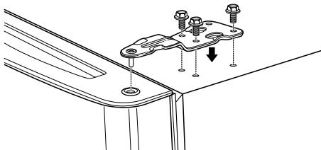
**2** Place the top hinge on top of the freezer door and line up the hinge with the holes on top of the refrigerator. Use the three bolts to fasten the hinge.
