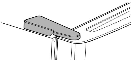
**5** Insert the decorative cover on the top right of the cabinet to cover the holes. Cover is force-fitted.
