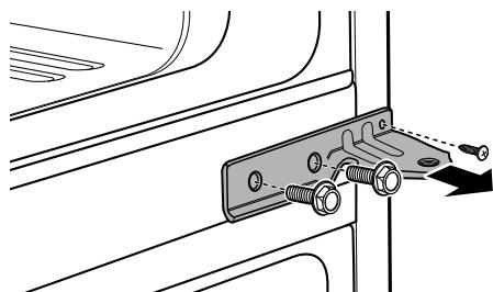
**4** Using a 1/4 in. socket wrench, loosen and remove the bottom hinge pin **4** from the bottom hinge bracket **5**. Remove the washer from the bottom hinge pin and set it aside.
