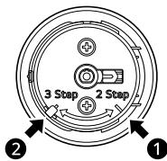
**3** Once the Knob Lock is adjusted as desired, reinstall the knob. To reinstall, hold the knob with the **OFF** label at the top and slide the knob directly onto the stem.
