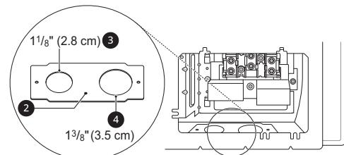
For power cord **5** installations, hook the strain relief over the 1 3/8 in. (3.5 cm) power cord hole located below the rear of the oven. Insert the power cord through the strain relief and tighten it.
