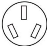
3-wire receptacle (10-50R)
