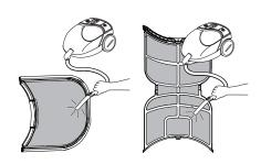
3 If the lint filter has become very dirty or clogged with fabric softener, wash the lint filter in warm, soapy water and allow it to dry thoroughly before reinstalling.
