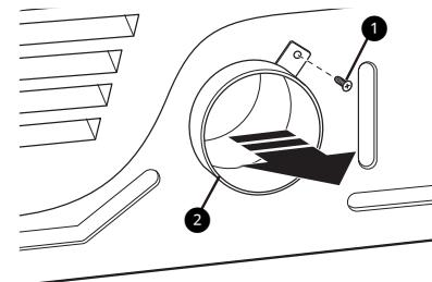
**2** Press the tabs on the knockout **3** and carefully remove the knockout for the desired vent opening. (Right-side venting is not available on gas models.) Press the adapter duct **4** onto the blower housing and secure to the base of the dryer as shown.
