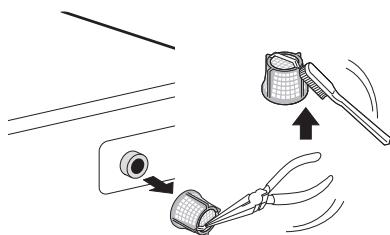
**5** Remove foreign objects and soak the filters in white vinegar or a lime scale remover.
