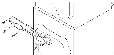
**3** Push open the caps at the left and right sides of the control panel on the front of the appliance. Loosen the screws under the caps.
