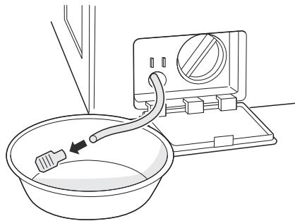
**4** Remove the pump filter.
