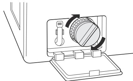
**8** Close the drain pump filter cover.
