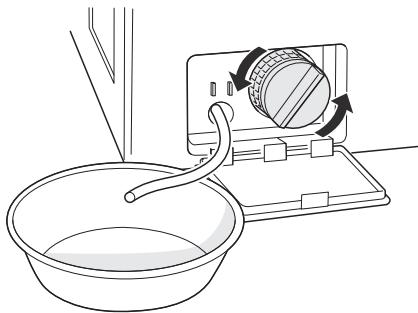
**5** Clean the pump filter and opening.
