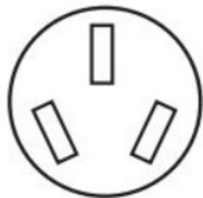
3-wire receptacle (10-50R)
