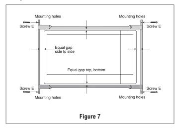
Install Air Deflectors top and bottom. Center (left and right) the Air Deflectors above and below the installed BACK FRAME. Secure AIR DEFLECTORS with 4 SCREWS E. See Figure 8. Mark holes and pre-drill the wood cleats with <sup>1</sup>/<sub>16</sub>" drill bit.
