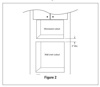
• The floor of the opening should be constructed of plywood strong enough to support the weight of the oven and floor load (about 100 lb/45 kg). The floor should be level and 90° with the face of the cabinet for proper installation and operation of the oven. Check the local building code that may require that the opening be enclosed with sides, ceiling and rear partition. The proper functioning of the oven does not require the enclosure.
