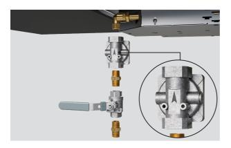
2. Ensure that the regulator arrow points towards the cooktop's inlet pipe, away from the gas supply.
