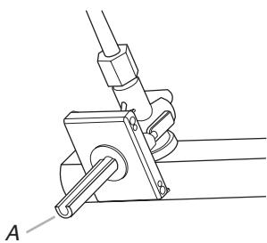
A. Valve stem on standard burner
