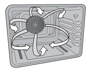
Figure 6: Convection roasting on lower oven racks
