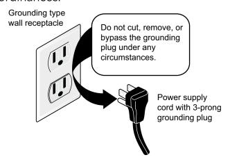
This appliance is equipped with a 3-prong grounding plug for your protection against shock hazard and should be plugged directly into a properly grounded receptacle. Do not cut or remove the grounding prong from this plug.
