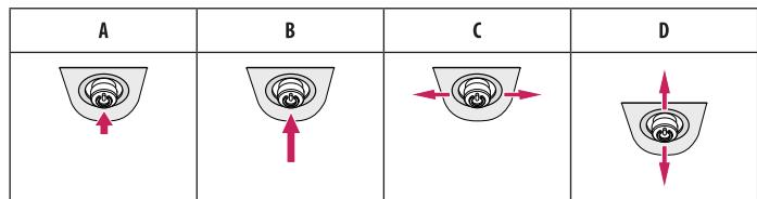
**A** (Power on): Press the joystick button once with your finger to turn on the monitor.
