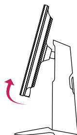
3 Rotate the monitor clockwise as shown in the figure.
