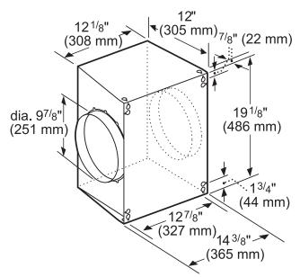
measurements in inches and mm
