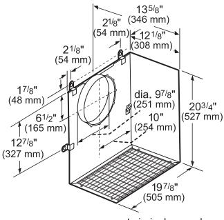
measurements in inches and mm
