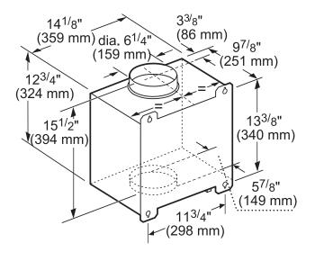
measurements in inches and mm
