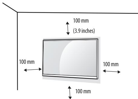
To install the monitor to a wall, attach a wall mount plate (optional) to the back of the monitor.
