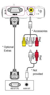
You can connect the audio cable without using a gender as shown in the illustration above.
