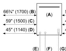
All connections are located on the rear of the appliance.
