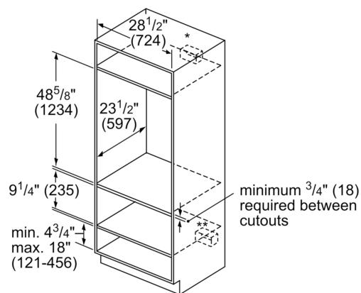
\* Wall oven junction box may be located above or right or left of the unit within reach of the power conduit.
