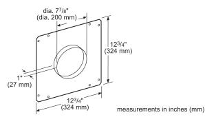
**NOTE:** HDDFTRAN6 or HDDFTRAN8 front plate required for front exhaust applications with inline and remote blowers.
